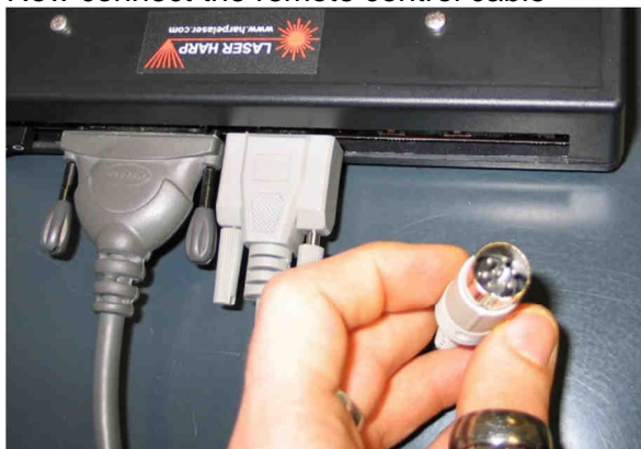
Connect the MIDI cable from the OUT connector of your synth to the IN of the controller
