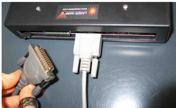
Connect the other end to your ILDA laser projector Now connect the remote control cable
