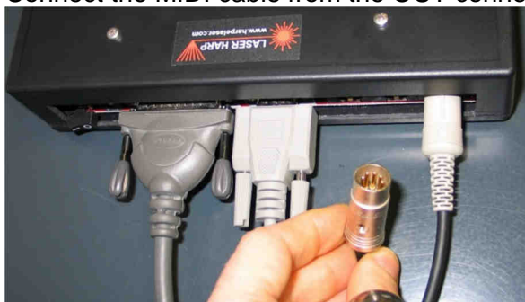
Connect the MIDI cable from the OUT connector of your synth to the IN of the controller
